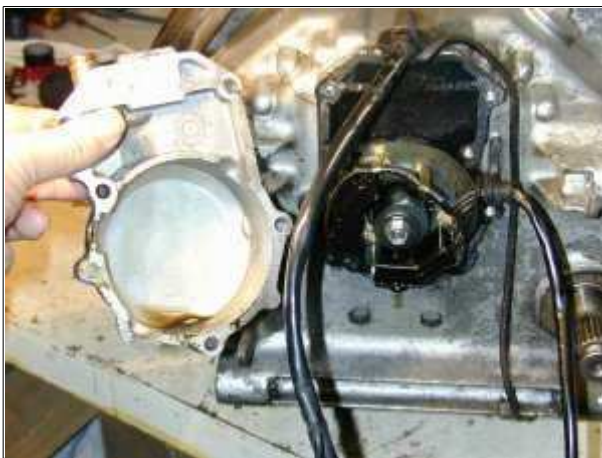
Ian says "This chrome water pipe bracket bolt did not want to come off, after drilling the top off the allen bolt."
