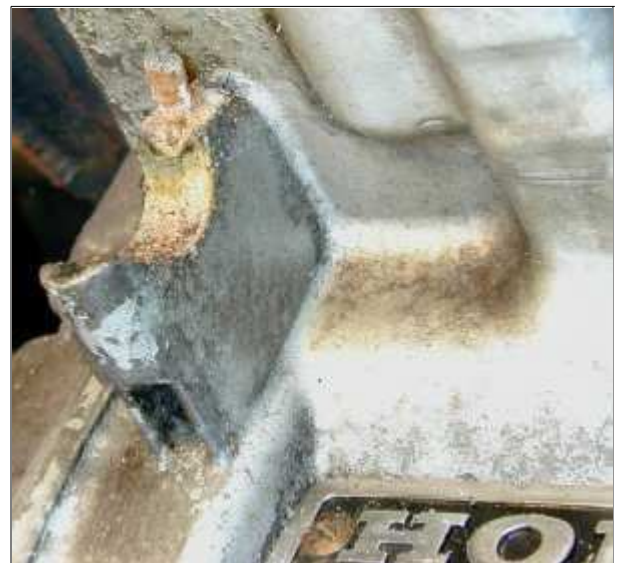
Ian says "This chrome water pipe bracket bolt did not want to come off, after drilling the top off the allen bolt."
