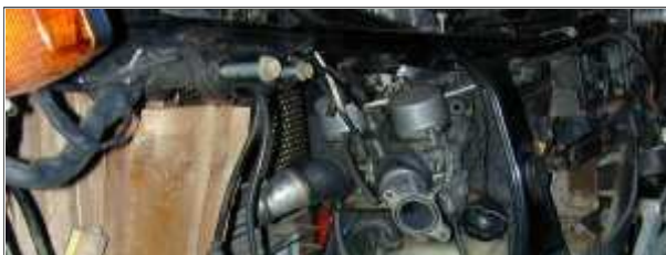
Eurosport frame after engine removal. Carbs are still fitted.
