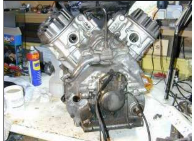
Rearmost small cover removed, showing the ignition sensors for transistorised ignition.
