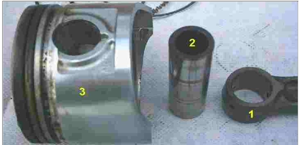
1 - connecting rod & little end. 2 - gudgeon pin (US: wrist pin). 3 - piston.
