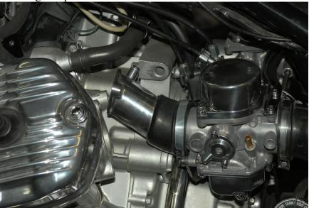
Now rotate the manifold back down into position and insert both bolts loosely to hold it in position.
