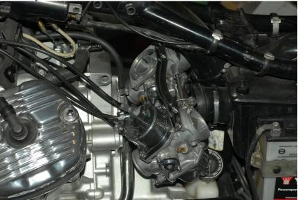
After they are in position, work them up into the air filter connections and clamp them lightly into position. Twist the throttle a few times to make sure your cables are not binding. Turn the bars all the way to the right to test this also. They seem to bind if they are not laid out right when the bike is turned to the right. The cables need to lay smoothly and not be twisted around each other, or have sharp bends in them. If it binds this is
