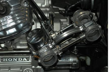
After they are adjusted with about 1/8" to 1/4" throttle free play, tighten down the lock nuts on each cable. Now turn the carbs with the top twisted to the front of the motor and gently work them in between the motor and the frame tube. You might need to move the wire harness a bit, but when positioned properly, they go in smoothly.
