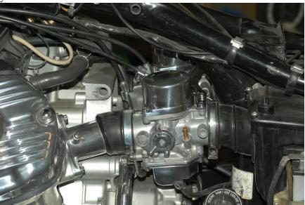
At this point I don't need to go into how to put on your tank and the fuel line. I will tell you though that you should always use a fuel filter of some kind. It saves a lot of frustrations when you all of a sudden end up with one side not idling or adjusting right because you allowed dirt and debris to get into a clean carb.
