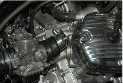
Now you can tighten up the intake manifold bolts, and all for clamps on the rubbers so they are secure and sealed. Make sure the air box fittings are lipped all the way around the intake side of the carb. They are a little hard to see some times. Use a flash light. Install the plastic ring in the top of the carb, LIP FACES UP.
