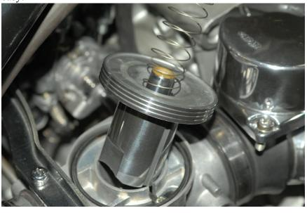
Secure the cover with it's 2 screws and attach the float bowl drain hoses.
