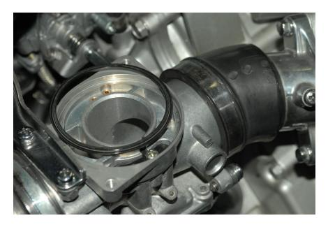
Then the piston and spring, be careful to align the slot up with the plastic guide, and be gentle with the slide needle. It should slide in easy.
