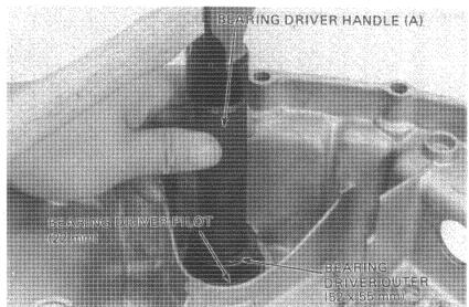
Install the final shaft oil seal and gear shift spindle oil seal.
