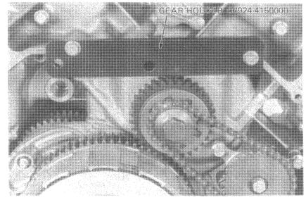
Remove the C.D.I. pulser rotor. Remove the flywheel bolt.
