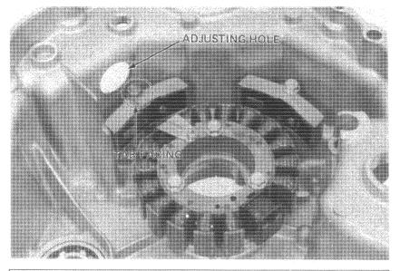
Install the C.D.I. pulser stator.
