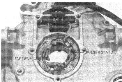
Remove the generator stator and right and left fixed pulsers.
